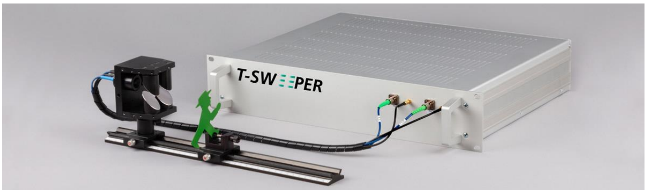
Figure 2. All-fiber terahertz spectrometer from FhG-HHI, operating at 1.5 \mu\text{m} optical wavelength with up to 70 traces per second and a bandwidth of 2 THz.
